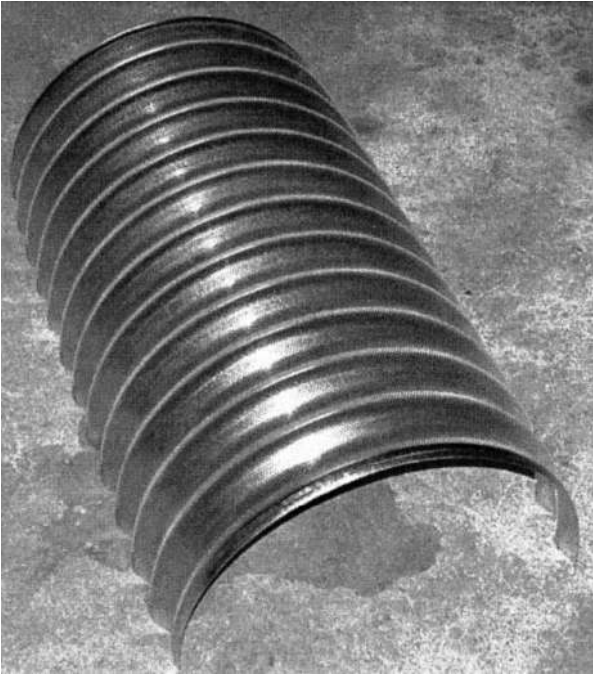
Imaginea 2 : Conducta de racire semirotunda (sistemul comparat)
